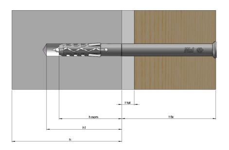
$h_1$  = depth of drill hole to deepest point
