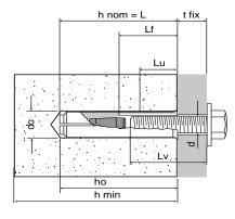
d screw diameter hole diameter do minimum support thickness hmin = hnom = nominal embedment depth cylindrical hole depth ho anchor length Lf anchor internal threaded length Lu minimum thread engagement metric screw / bolt length Lv
