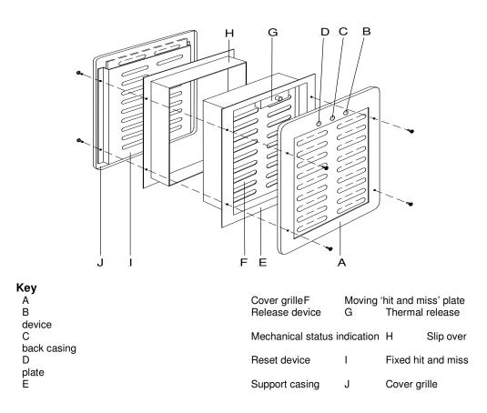
Figure 3 – Mechanical Air Transfer Grille (Type M and MMS similar)
